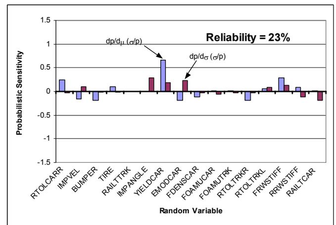
**Figure 11. Probabilistic Sensitivity Factors for the Original Design.**
