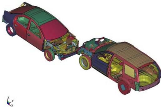
**Figure 3. Vehicle-to-Vehicle Frontal Offset Crash Simulation Model.**
