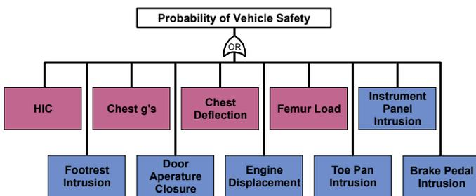
**Figure 10. Probabilistic Fault Tree of the Crashworthiness Model**
