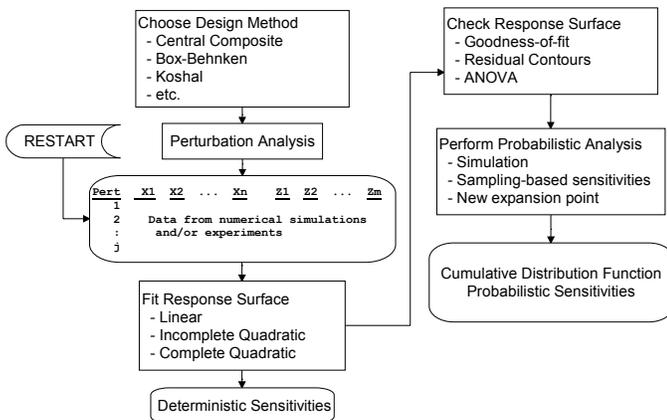
**Figure 2. Probabilistic Analysis using a Response Surface Model**
