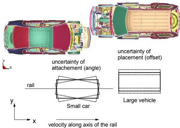
**Figure 5. Model Setup**
