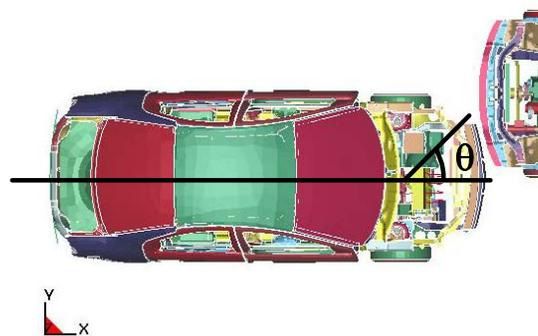
**Figure 9. Impact angle uncertainty is modeled by rotating the small car nodal coordinates around the CG.**
