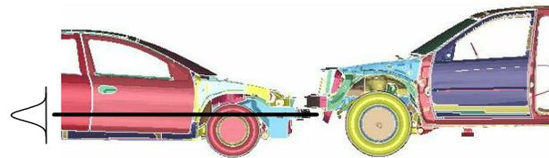
**Figure 8. Tire height uncertainty is modeled by moving the small car nodal coordinates in the Z direction (distribution is not to scale)**
