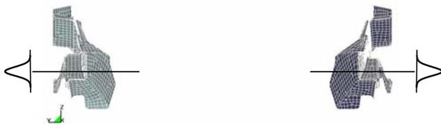
**Figure 6. Left and right small car rails with assembly uncertainty are modeled as two random variables.**
