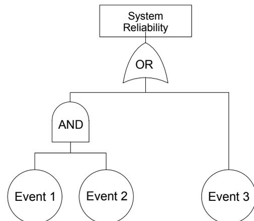
**Figure 1. Example of a Fault Tree for System Reliability Analysis in NESSUS**
